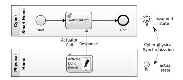
Fig. 1. Scenario Process Showing the Synchronization of Cyber and Physical Worlds.
